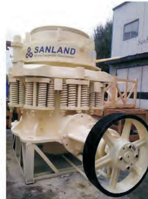
The Sanland-made cone crusher is a U.S. licensed product with all its spare parts to be interchangeable with the original American Symons cone crushers;
