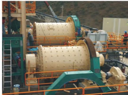
Ball mills are composed of such major parts as feeding, discharging, revolving and driving parts (reduction gear, small driving gear, electric motor and electric control), The hollow shaft is made with steel casting with available lining replacement and the rotating big gear is made with casting and hobbing technique. There is abrasion-resistant lining inside the barrel. Therefore, the ball mill has high abrasion-resistance, smooth operation and reliable performance.
